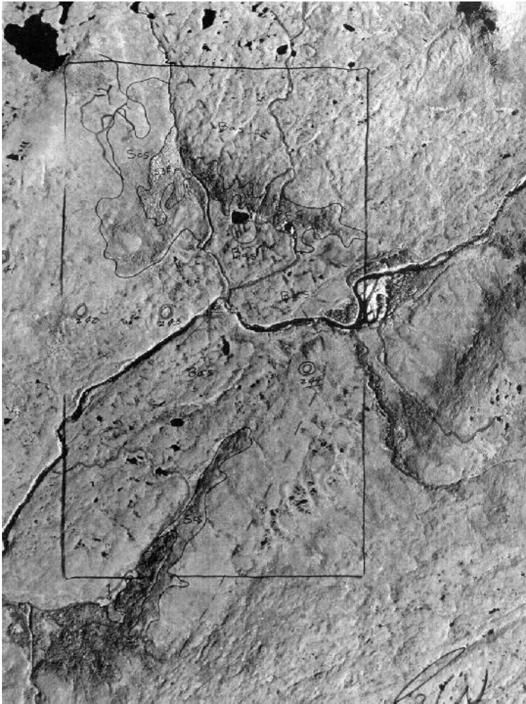
Figure 17. Air photo of the Burgeo barrens taken before the highway was built. The dashed pencil line marks the route of the highway. Sites 44a and 44b are located on either side of the highway, respectively, where it passes over the escarpment beside the small pond due north of the sharp bend in the river on the left.
